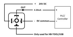
**Note:** Special USB cable and adaptor/converter plug is needed for scaling the temperature measuring range.
